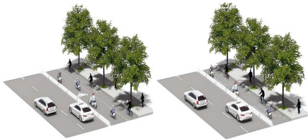
Figure 37. Share lanes for both bicycles and motorized vehicles (Source: WRI, 2021)
