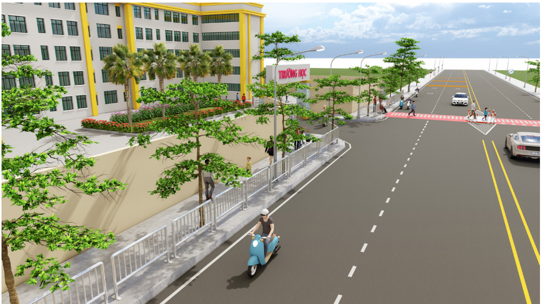
Figure 41. Safety guardrails on sidewalks in school zones
