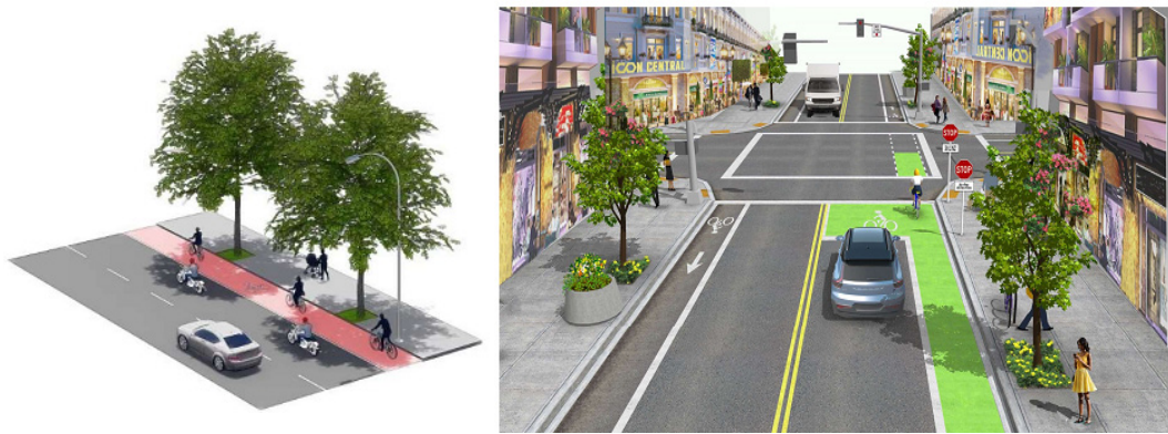
Figure 38. Pavement design of bike lanes (Source: WRI, 2021)
