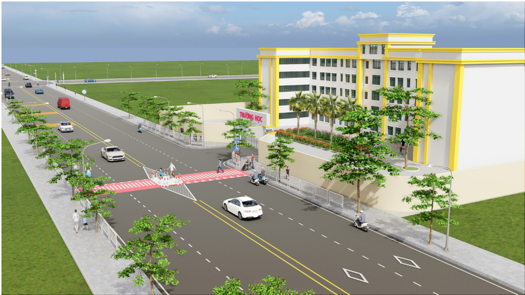
Figure 40. Design of sidewalks in a school zone
